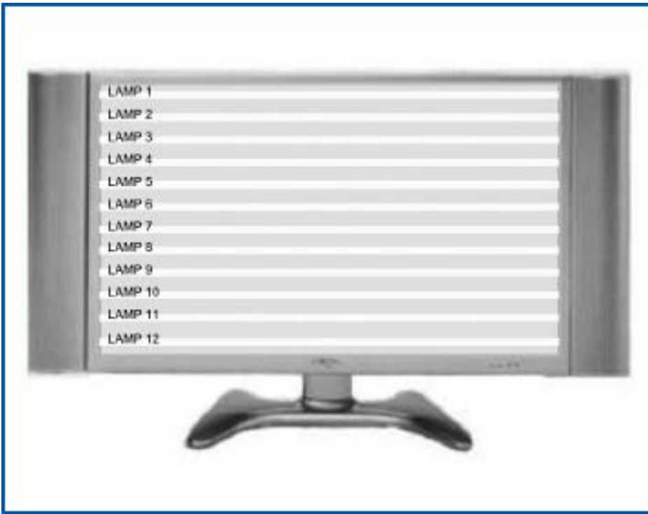
Figure 12. LCD TVs contain from 4 to 40 CCFLs.
